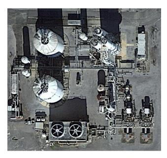
The plant has a film-type main vaporizer with two BAHX closed cores supplied by Sumitomo and is equipped with an alumina/CaBaX air purification system.
